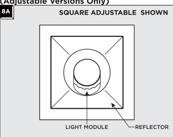
1 Using your fingers, adjust the direction of the light making sure to turn the module not the reflector (see note below).
