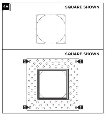
2 Install the provided 6x20 self-drilling screws through the plaster plate and housing at the marked locations. Do not place screws at any of the other mud holes on the plate.
