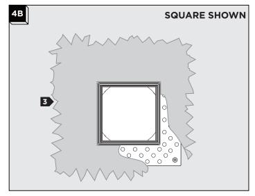
3 Properly plaster onto the plaster ring and drywall.
