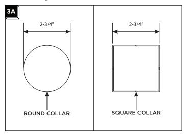
Mark an appropriate sized diameter circle or square on drywall. Cut out the marked section. **Note:** The drywall may be cut by running a 1/8" RotoZip around the outside of the collar.
